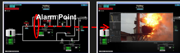
Alert Validation and Data Correlation by SCADA/IDS/LDS/SENSOR linkage with IVS
